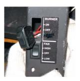
9) Connect the female connecter on the white wire to the TH terminal of the valve.
